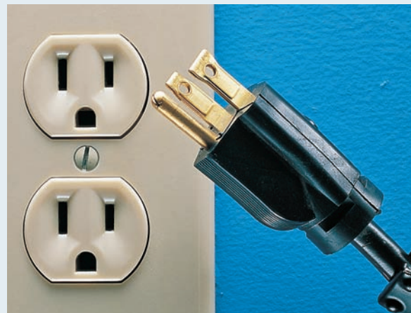
Three-slot receptacles are required by code for all new installations. They are usually connected to a standard two-wire cable with ground.
