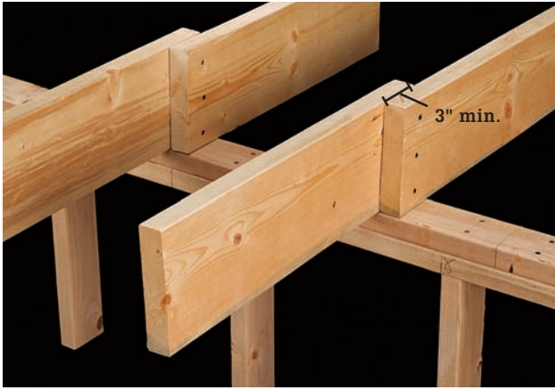
Lap joists that meet over supports with at least 3" overlap. Reinforce the lap joint with at least three 10d nails.
