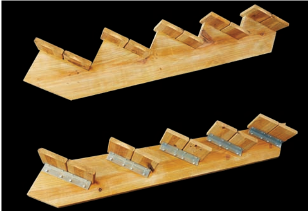
Cut stringers (top) should be supported every 6 feet. Solid stringers (bottom) should be supported every 13 ft. to 3".
