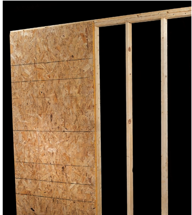
Wood structural panel wall bracing may be used on all stories and in all seismic and wind design areas.
