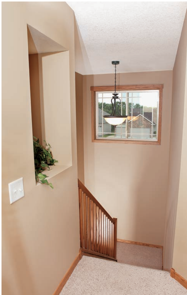
One light at a center landing may not be enough to illuminate the top and bottom landings.
