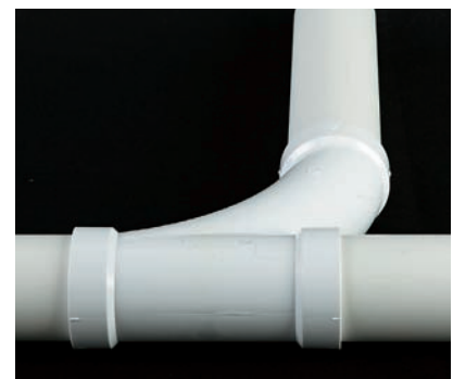
Changing flow direction from horizontal to horizontal using a long-radius tee-wye fitting.
