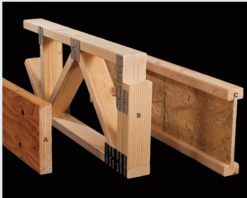
Beam types: Laminated beam (A), web-type truss, metal plate connected (B), I-beam joist (C).
