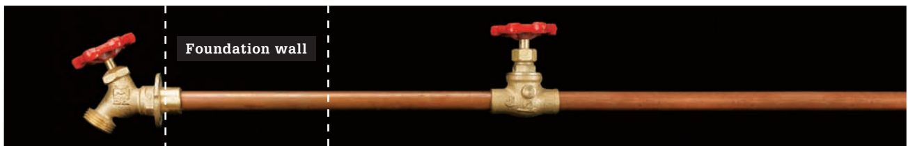
Hose bibbs that are subject to freezing require a stop-and-waste valve inside the building.
