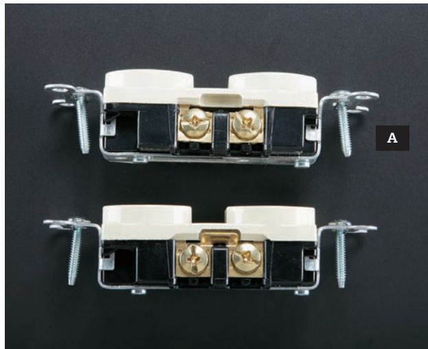
The receptacle yoke is removed (A) when it is split-wired using a multiwire branch circuit.
