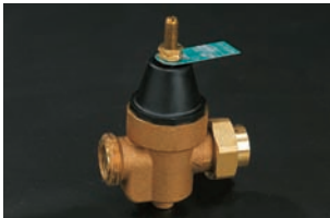
Install a pressure-reducing valve when the water pressure exceeds 80 psi.
